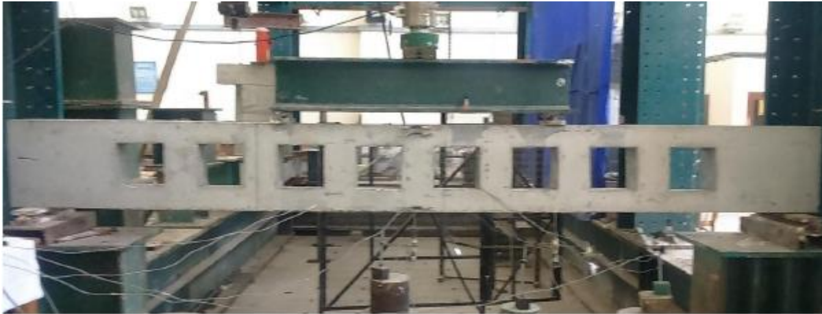
Fig. 2: Test setup and instruments.
