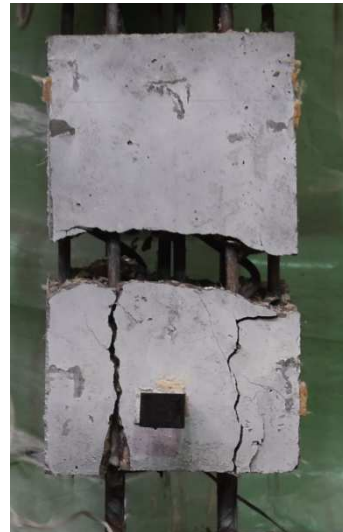
(b) slippage of outer linking bars of G1-SO-10d.
