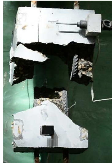
(b) Front face of G2-H-10d showing direct shear plane of failure
