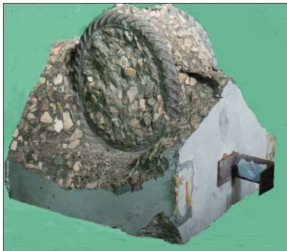
(a) side view of G2-H-10d showing direct shear plane of failure
