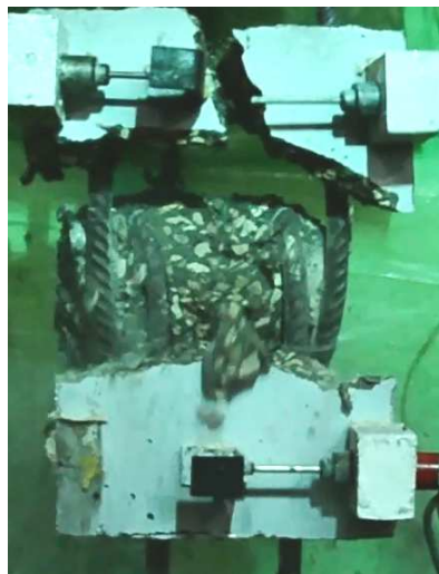
Fig. 13 concrete block formed after failure of G2-HC-10d.
