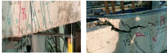
Fig. 9C: the mode of failure for Specimen B1
