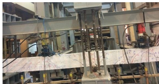
Fig.9a: Control Specimen Ao crack pattern
