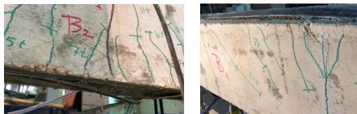
Fig.9E: the mode of failure for Specimen B2
