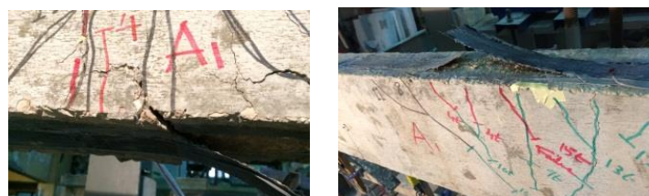
Fig.9a: Control Specimen Ao crack pattern
