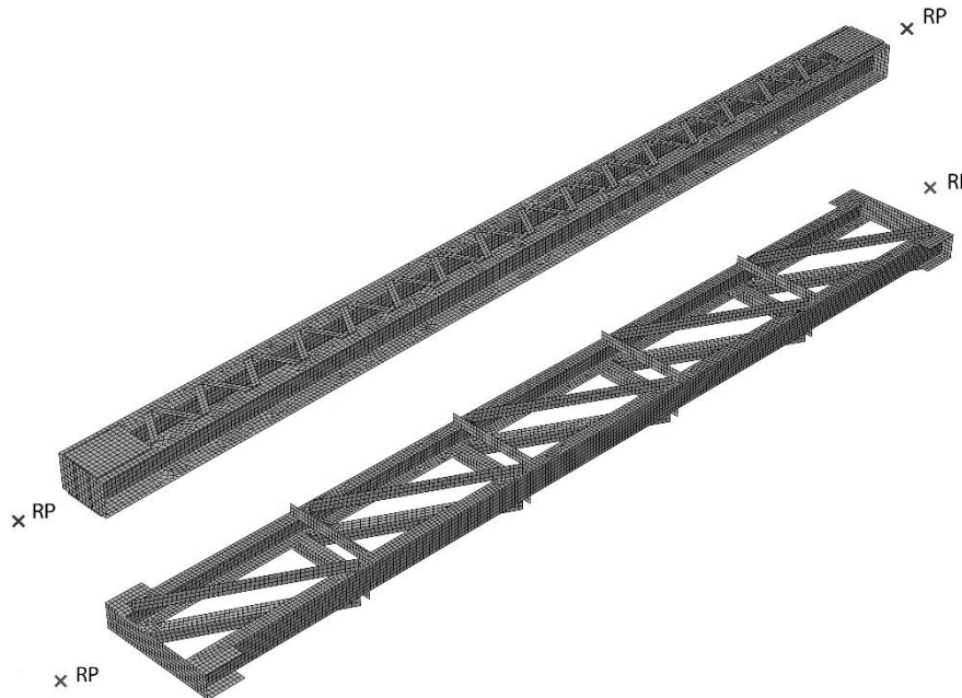
Fig. 3: Current finite element mesh for axially and eccentrically loaded columns
