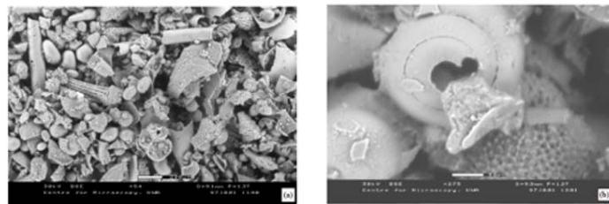
Fig. (2): SEM micrograph for GW soil: (a) angular particles with different and (b) hollow fragile particles (after Ismail, 2000)
