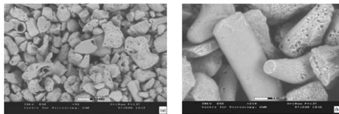
Fig. (3): SEM micrograph for LP soil: (a) particles with different origin (b) close up view of the particles showing rounded edges with high aspect ratio (after Ismail, 2000)
