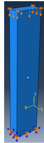
Fig.5 Loading and defined boundary conditions places.
