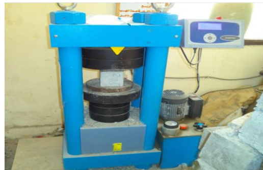
Fig. (8) Compressive strength testing machine
