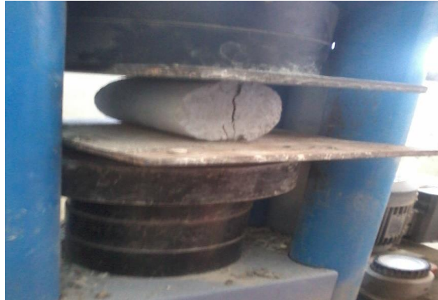
Fig. (15) Splitting tensile strength testing machine
