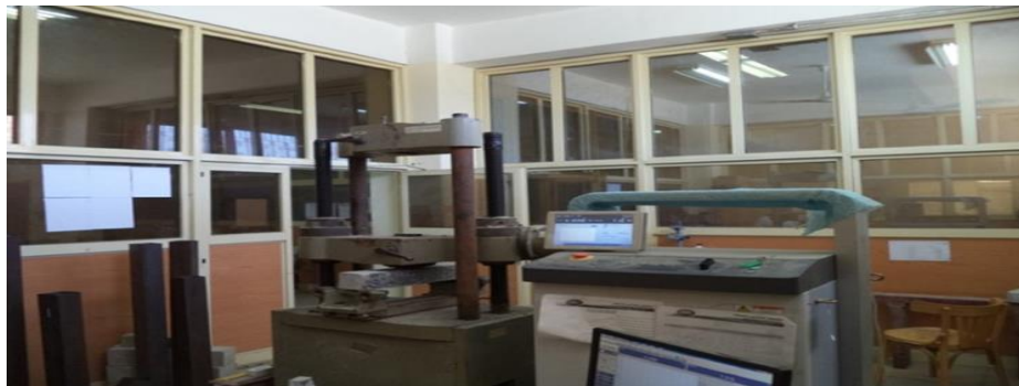
Fig. (19): Universal testing machine (300 KN) for testing specimen under flexural
