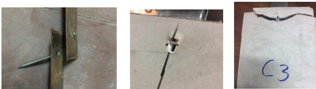
Figure 3 Modes of failure in the three screw connections in Steel, Cement and Gypsum board
