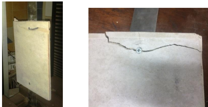
Figure 8 FCB test configuration and failure modes during shear loading test
