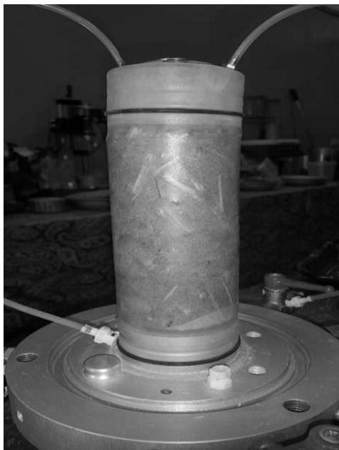
Fig.3.a: Soil sample (S8) in triaxial cell
