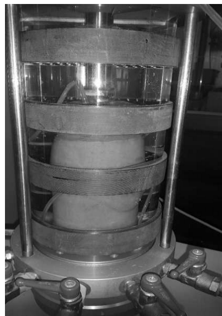
Fig. 3.b: Shear failure in Soil sample (S1)
