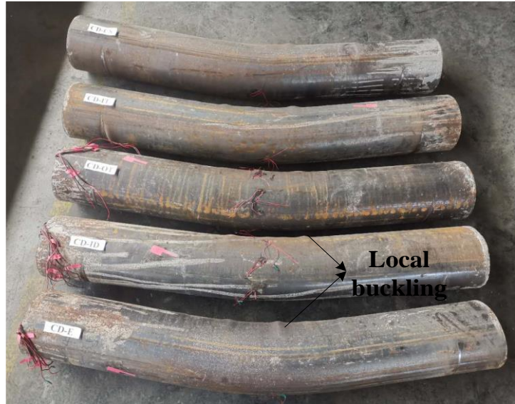
Fig. 4: Failure modes of CFDST specimens.
