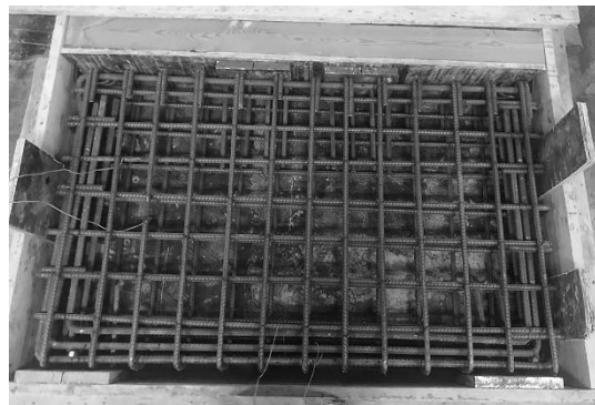
Fig. 3: reinforcements details of the tested beams.
