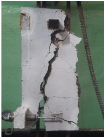
Fig. 5 Bars pullout of G1-O-20d.
